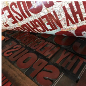
The poster being printed from the wood-block letters of the letterpress. (Pete Morelewicz)
